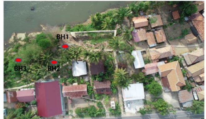
Figure 1. Research location and soil testing sample points
